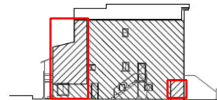
NORTH ELEVATION ALONG PROPERTY LINE (R = 1,127 SQ FT, D = 270 SQ FT)
